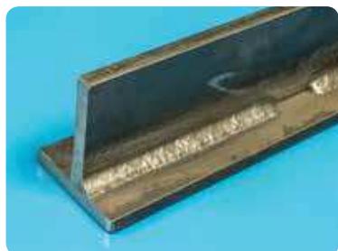
Clean weld surface
